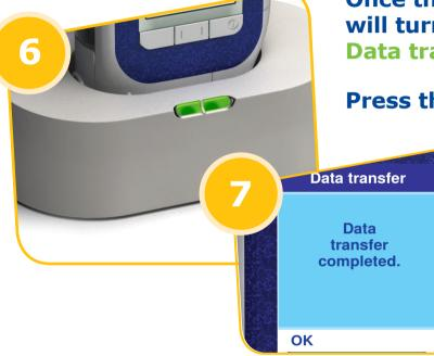
Once the upload is complete, both lights will turn green and the device will read: Data transfer completed.
