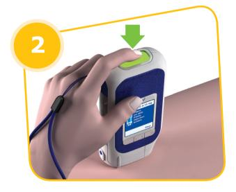
When the easypod is properly positioned against the skin, the injection button turns green and the easypod will beep once.
